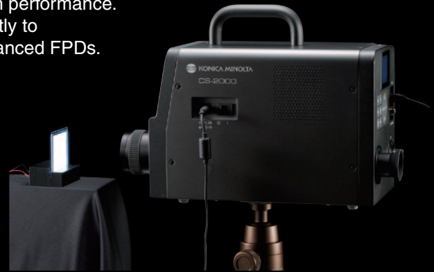
Measurement example: Measurement of an organic EL illumination panel during development
